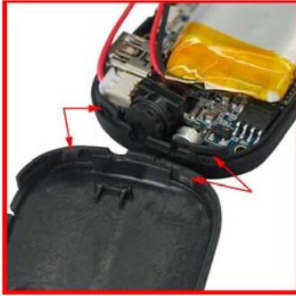
(1) Note the two latches inside the case.
